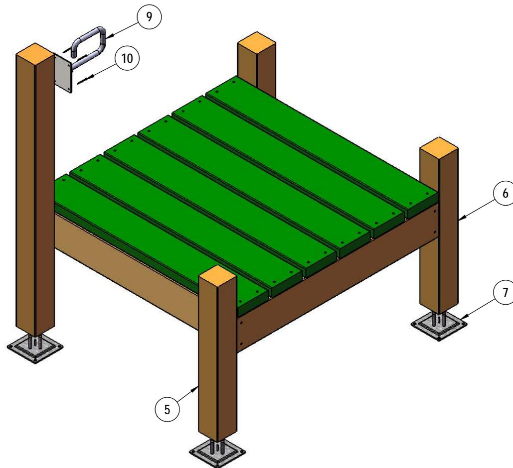
Attach the Surface Mount Plates to the bottom of the Left and Right 4" x 4" Posts with the included mounting hardware.
