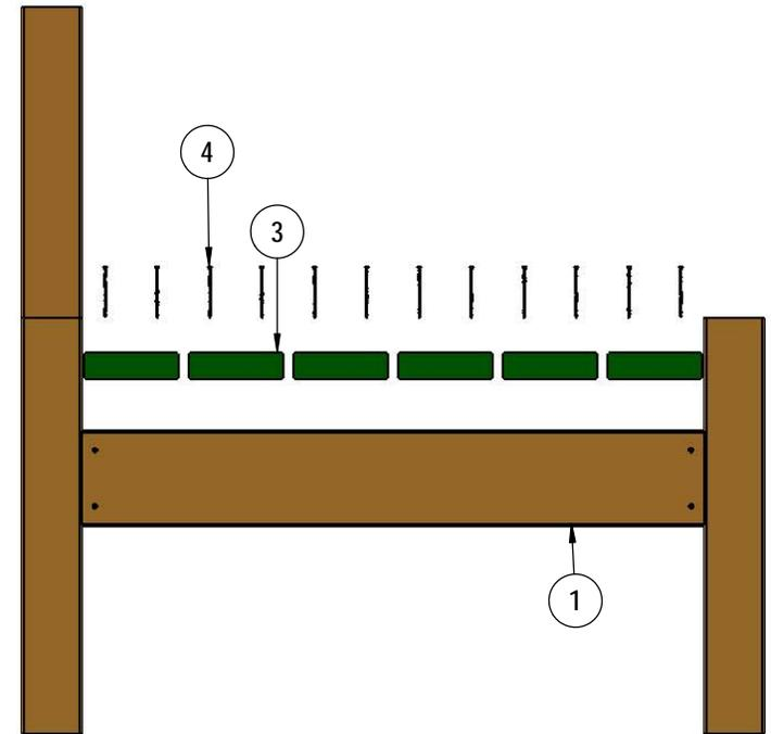
Attach the 2" x 6" x 36" Green Recycled Top Planks to the 2" x 6" x 36" Cedar Planks using the specified hardware.
