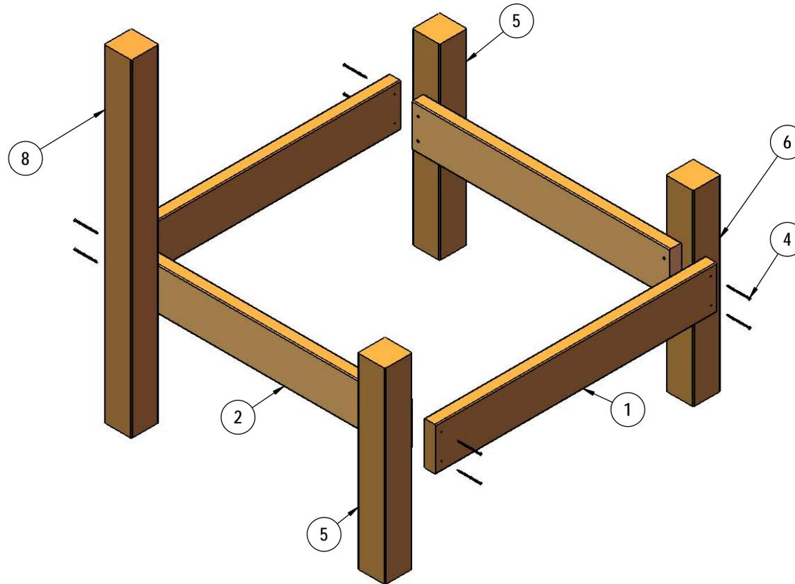
Attach the 2" x 6" x 36" Cedar Recycled Planks to the ends of the 2" x 6" x 33" Cedar Recycled Planks using the specified hardware.
