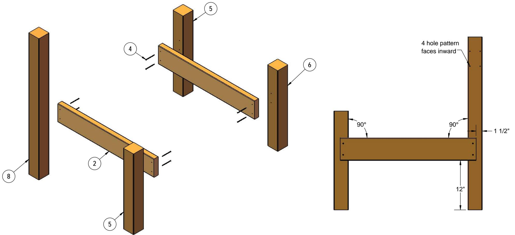
Attach the 2" x 6" x 33" Cedar Recycled Planks to the Left and Right Legs using the specified hardware.
